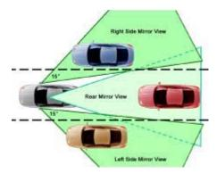
Traditional settings overlap with the rearview mirror view and should only be used if the view of the highway from the inside rear-view mirror is blocked.
