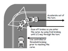
The vehicle's speed and load, and the sharpness and bank of the curve effect vehicle control. Traction loss when entering a curve is often caused by excessive speed, braking, or steering. Front tire traction loss is referred to as "under-steer," and is more likely to occur in front-wheel drive vehicles. "Over-steer" is when there is traction loss by the rear tires and occurs more often in vehicles with rear-wheel drive.
